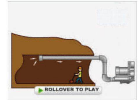
Tunnel engineering ventilation
